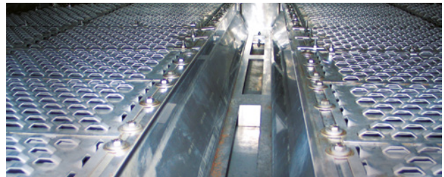
2-pass VG AF trays with V-Grid, sloped outlet weir and push valves.
