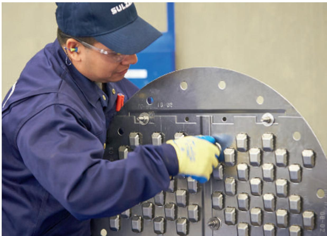
valve (Fig. 1), that substantially improves all three main performance characteristics of the fractionation tray: mass transfer efficiency, hydraulic capacity, and operating range.
