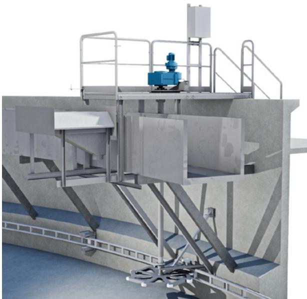
The scraper can be equipped with a peripheral surface scraper, supported from the bottom scraper arm. The surface scraper collects the surface foam in the scum box unit which is attached to the concrete wall. The sludge is removed from the scum box through pipes in the concrete wall.
