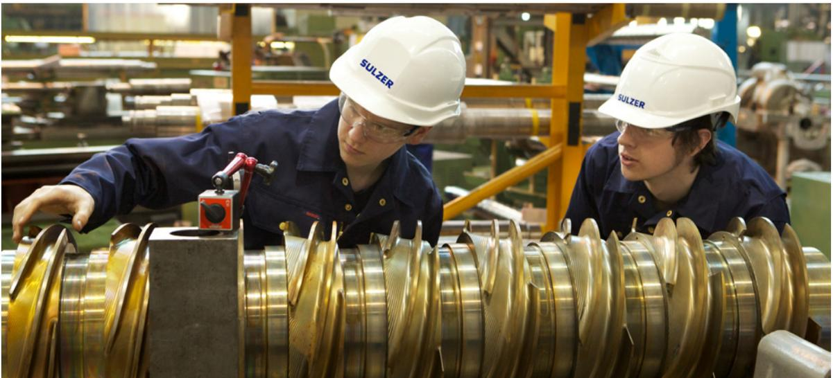
Dunbar multiphase pump rotor on the balancing machine
