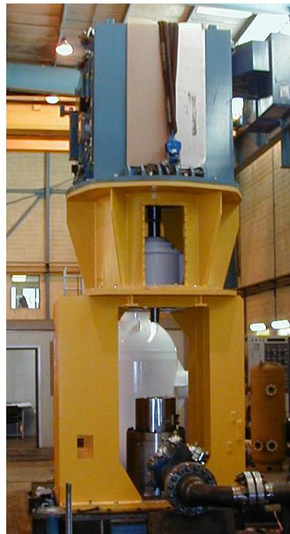
Dunbar multiphase pump package during Factory Acceptance Test (FAT)
