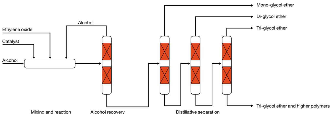
4<sup>■</sup> The manufacture of glycol ether is conducted in three main stages: mixing and reaction, alcohol recovery as well as the separation of the end products in a three-stage distillation. The key components developed by Sulzer Chemtech are employed in all three stages.
