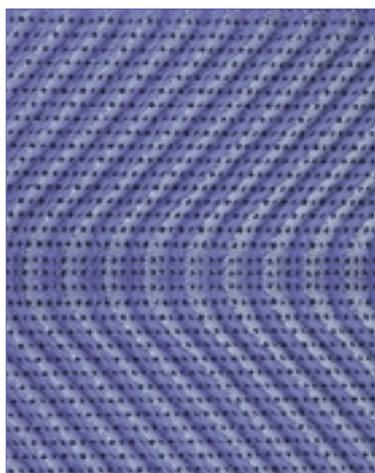
5<sup>■</sup> Since the metal packing from Sulzer Chemtech (photo: MellapakPlus) cause only extremely low pressure losses, the distillation can take place at low temperatures. This increases the purity and quality of the separated glycol ethers.
