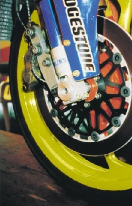
2<sup>■</sup> The brake fluid in hydraulic brakes (with glycol ether as the main constituent) transfers the brake effort from the brake cylinder to the brake block in a uniform manner. The fluid must have a high boiling point and is not allowed to attack the brake-line materials or the seals.
