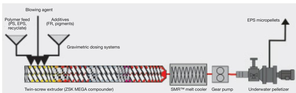
[3] Sulzer's EPS process is suited for small-scale EPS production (500–3000 kg/h).
