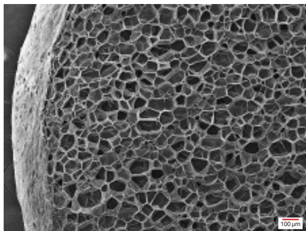
2 Prefoamed EPS beads from Sulzer's EPS process show excellent sphericity and cell size distribution.
