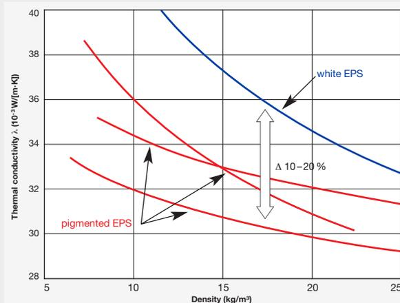
1 Adding pigments decreases the heat conductivity λ and improves the insulative properties of the EPS. This kind of “low-lambda” development allows access to markets for high-performance insulation materials.
