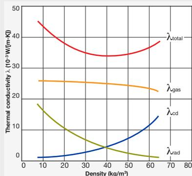
The thermal conductivity κ or λ (measured in watts per meter kelvin W/(m·K)) describes the ability of materials to conduct heat.
