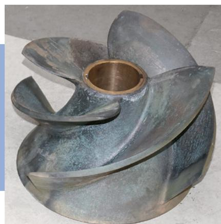
Ruedi Stöckli is responsible for the inspection and overhaul of the pumps. His team has just dismantled a Sulzer pump built in 1958. Despite its advanced age, the impellers are still in good shape.
