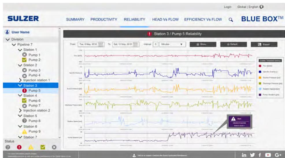
Fig. 5 Correlation of pump data with warning at vibration threshold.
