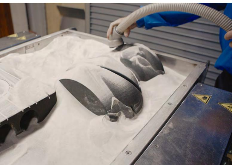
Fig. 2 Creating new components using sand for a 3D printed mold.
