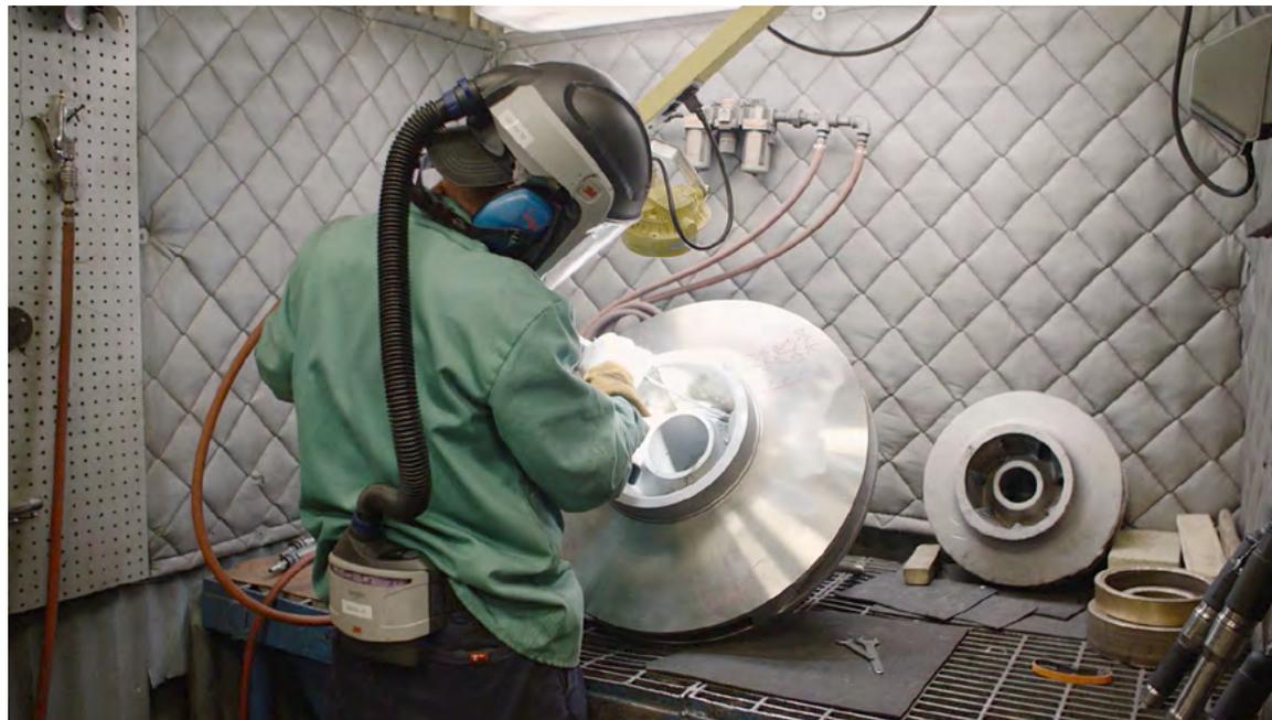
Fig. 4 Specialist cleaning and polishing equipment complete the process.
