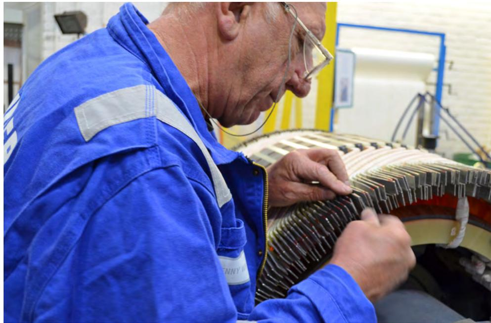
Fig. 4 The damaged components were rewound while the investigation into the cause progressed.
