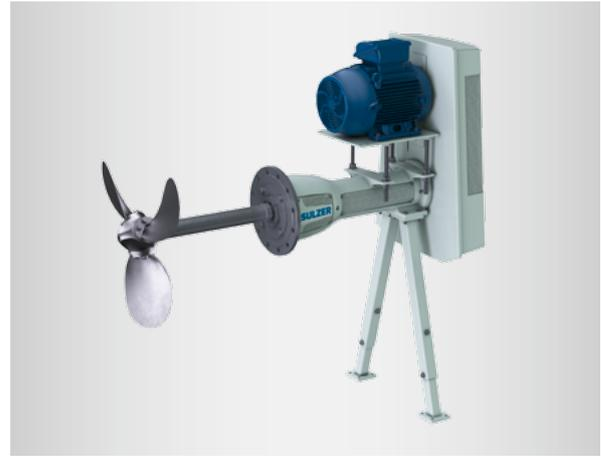
This ensures a longer lifetime than for agitators using austenitic stainless steel propellers. In addition, the performance of the agitator can be adapted with the adjustable propeller blades. The EX3 propeller is so extremely efficient, that Sulzer decided to offer it as a retrofit set for older MX4 propellers as well.
