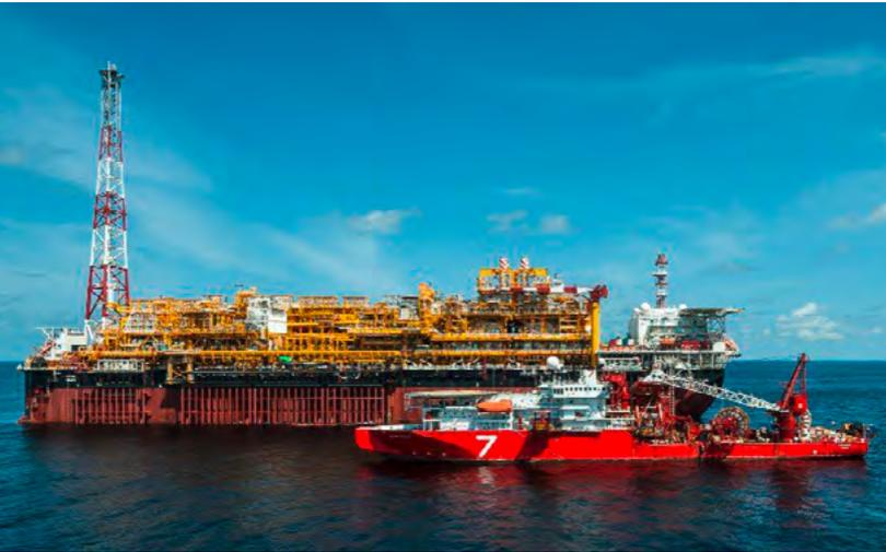
1 The CLOV FPSO is using the Total-patented wash tank technology.
