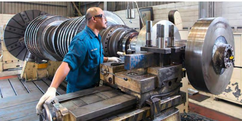
3 The HPIP rotor required extensive weld buildup and machining to deliver nominal dimensions.
