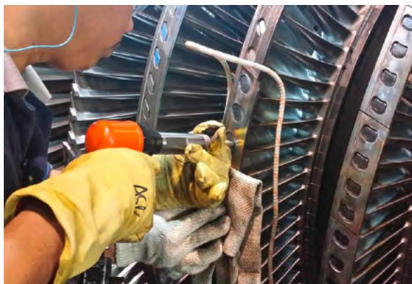
6 New HPIP rotor blades were installed and secured with a hot peening process.
