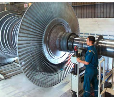
5 Low-speed balancing of all components before shipping.
