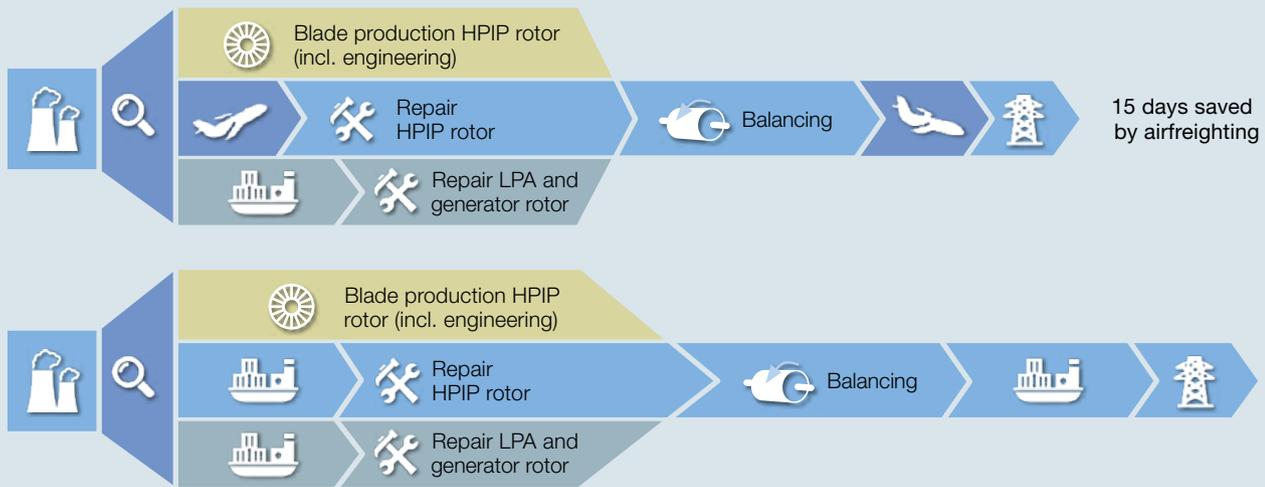
2 The repair with parallel workflows and rapid transport took 85 days only – 15 days were saved by airfreighting.
