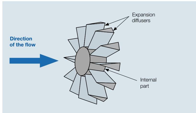
2 The EcoSpand expansion diffusers in the gas duct separate the gas stream.
