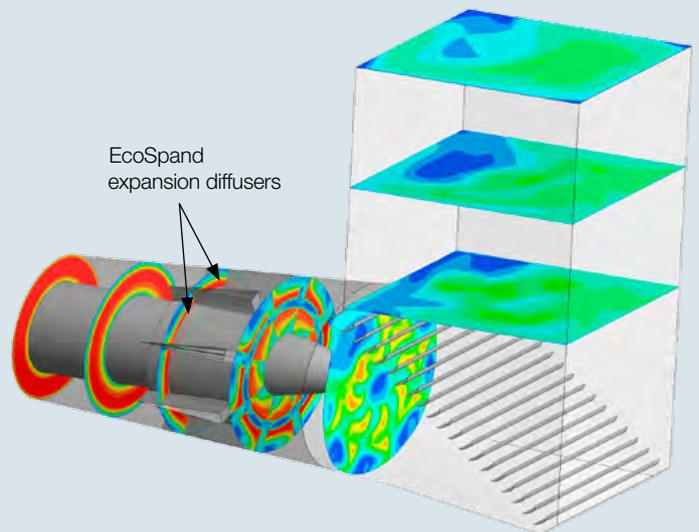
3 CFD analysis of the distribution of the velocity in the gas duct (left without EcoSpand / right with EcoSpand).
