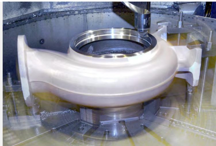
4 Processing of a pump casing from duplex stainless steel.
