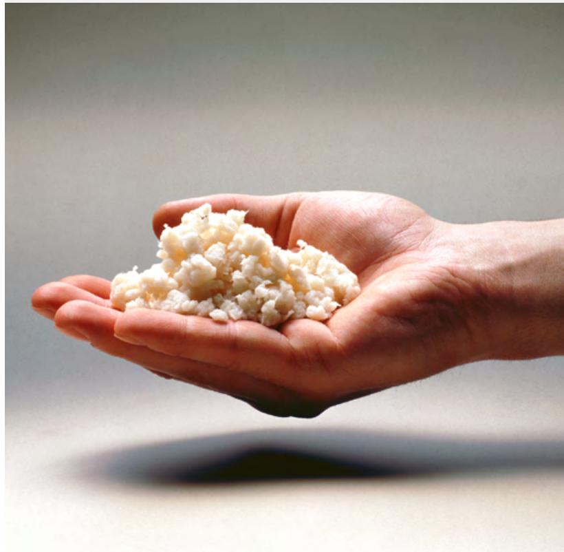
2 Medium consistency pulp contains fiber, water, and air.
