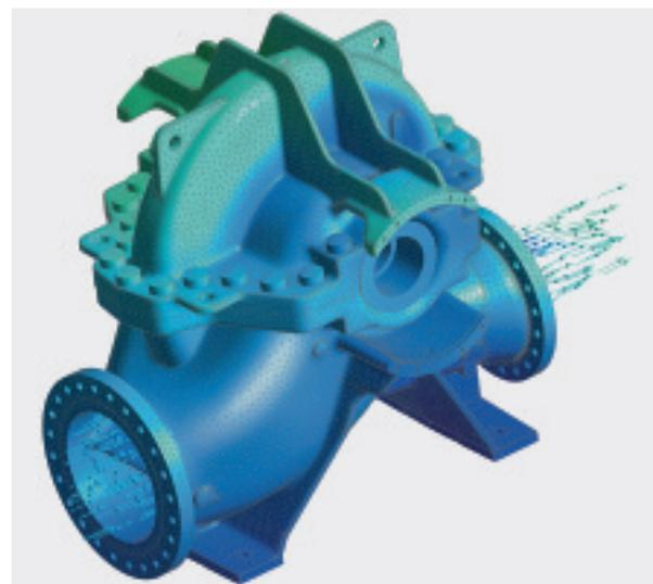
3 Finite element analysis (FEA) was used during the design process to ensure mechanical integrity.
