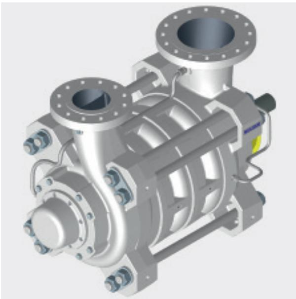
6 The new MBN-RO multistage ring section pump has special suction impeller for low NPSH<sub>a</sub>, as well as high-quality cast impellers and stage casings for better efficiency.
