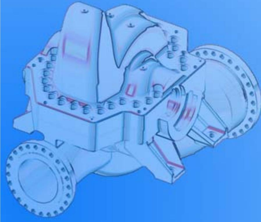
▶ The HPDM 600-940-s+s/30 pump produces approximately 9 MW in power. The finished casing weighs 26 tons and consists of a horizontally divided casing that is held together by studs (Fig. 1). In a typical two-stage pump of this kind, the two impellers are arranged back-to-back, which minimizes the axial thrust on the shaft. During the design phase, particular attention is paid to the adaptation of the casing to the internal pressure.
