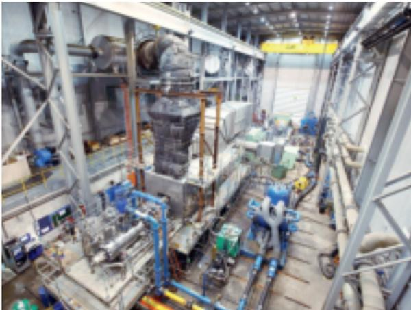
This development test bed is part of the development process for new products or pump ranges as well as of special large engineered pumps. The hydraulics group in Switzerland has significantly contributed to the design of new pump ranges with a greenfield approach. For example, the model testing in Winterthur verified the CFD analysis and hydraulic design of pumps developed for a new pipeline in Eastern Asia.
