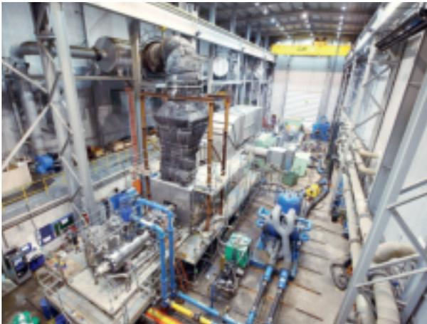
ment as a function of suction pressure or NPSH. For this purpose, model pumps are equipped with large windows allowing visual access to the entire eye of the suction impeller over 360°. Sulzer Pumps uses the high competencies of Sulzer Innotec in complex NC machining for the production of these model pumps. These skills are needed to successfully machine the complex 3D contours of casings and impellers out of solid blocks of aluminum.
