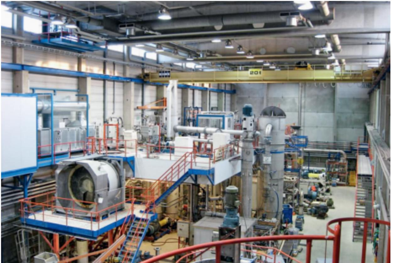
year, the test setup needs to be standardized with a high turnover. The required rapid setup and breakdown is achieved with modular pump interface piping that can be quickly rotated into position using custom-built rotating assemblies holding the required range of suction and discharge pipe sizes.
