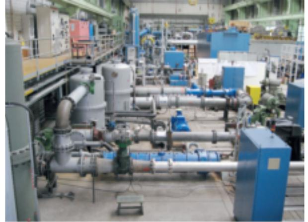
[3] With seven singular test loops, the test bed in Oberwinterthur is highly flexible.
