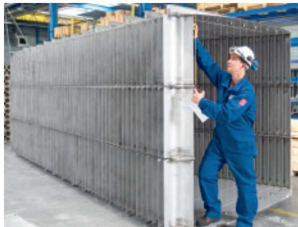
1 The conventional Schoepentoeter is one of the most effective devices available on the market for a bulk gas-liquid separation, where generally no more than 95% of the liquid needs to be removed from the gas stream.
