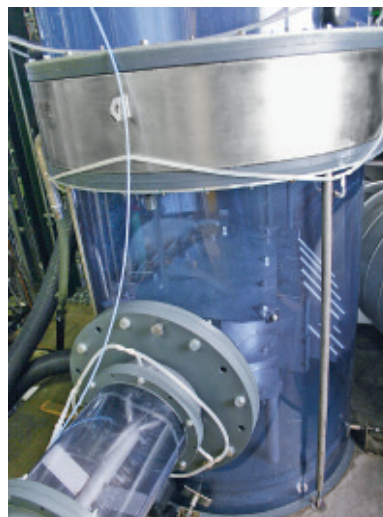
2 Several experiments were carried out at the Sulzer Chemtech pilot plant in Winterthur and at the Shell Technology Center in Amsterdam. The picture shows a pilot column in operation.
