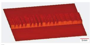
4 Three-dimensional pictures of erosion damage caused by water jet.
