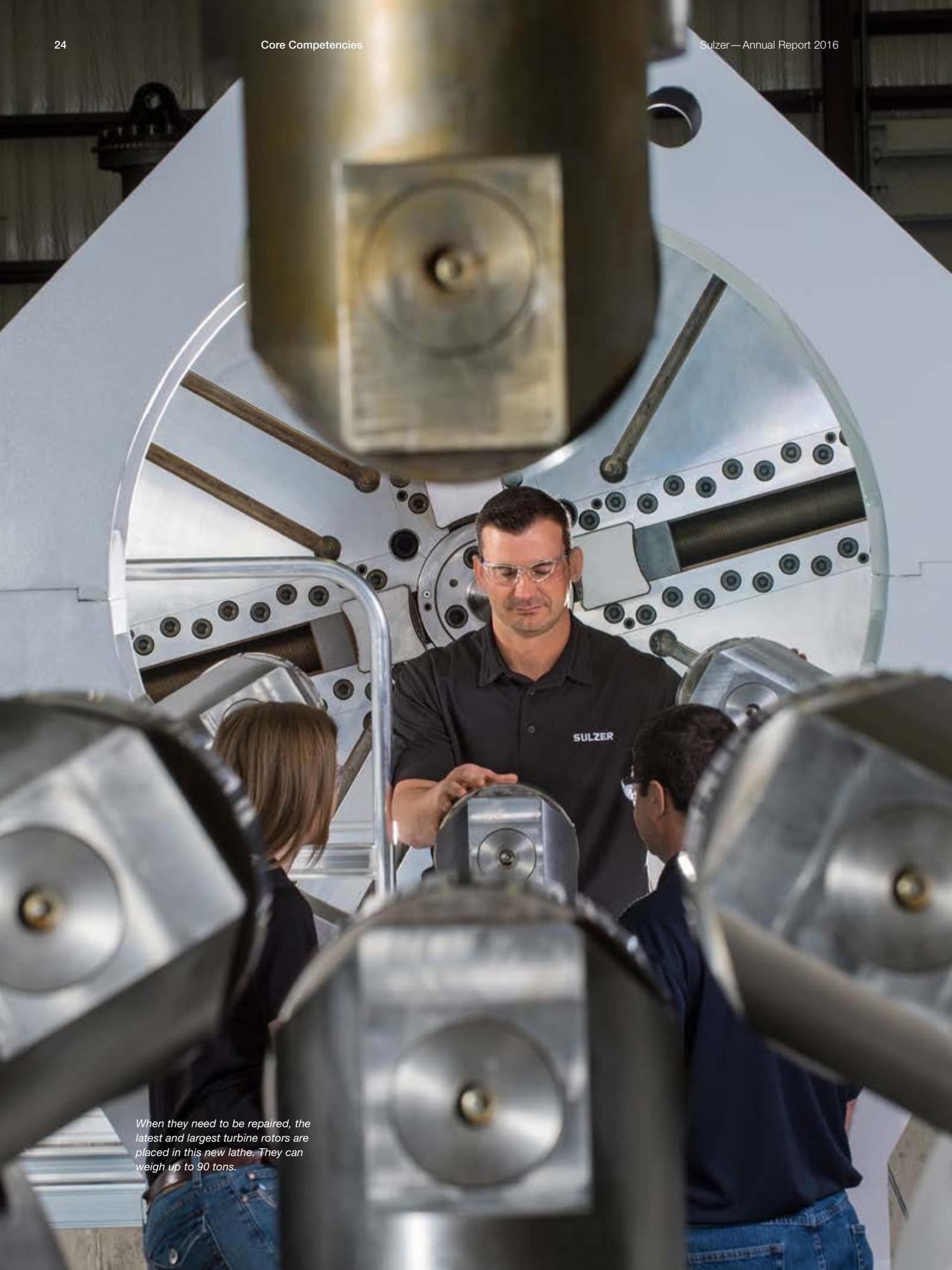
*When they need to be repaired, the latest and largest turbine rotors are placed in this new lathe. They can weigh up to 90 tons.*
