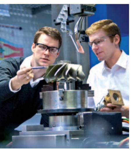
Sulzer Innotec developed a mobile high-precision laser system, which allows metal forming with five axes simultaneously.
