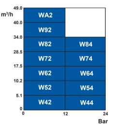
m³/h = capacity. Bar = differential pressure.
