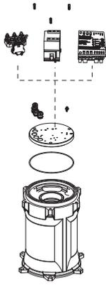
Figure 26: Mounting of terminal plate (J 205)
