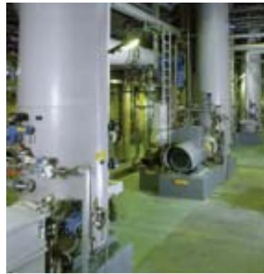
4 Typical MC<sup>®</sup> pumping arrangements. The stock level in the dropleg is measured and controlled, thus providing constant operating conditions for the pump.
