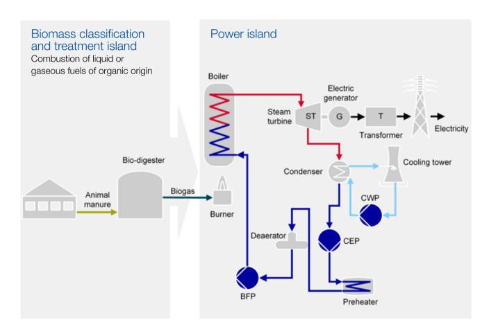
BFP = Boiler Feed Pump
