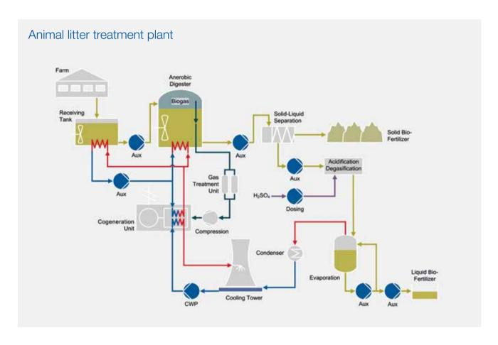
CWP = Cooling Water Pump Aux = Auxiliary Pump
