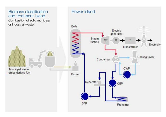
BFP = Boiler Feed Pump
