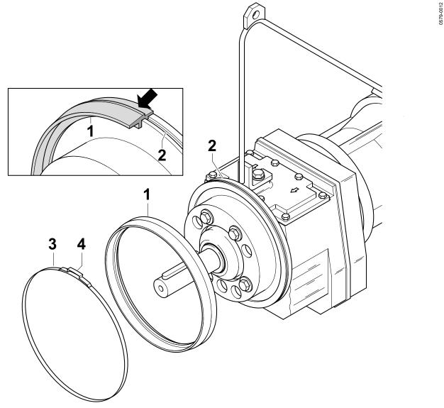
Figure 19 SD-ring removal/assembly
