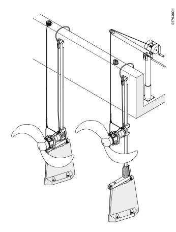
Figure 1 SB with self-adjusting coupling system (old System)
