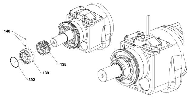
Figure 15 Assembling of the mechanical seal XSB 2750
