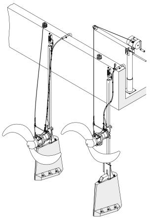
Figure 2 SB/XSB with lockable coupling system
