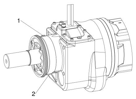
Figure 18 Oil filling and oil change XSB
