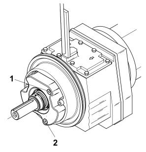
Figure 17 Oil filling and oil change SB
