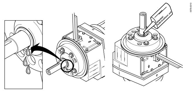
Figure 16 Oil filling and oil change
