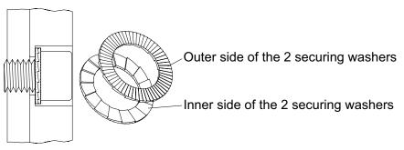
Figure 5 Correct fitting position of the Nord-Lock<sup>®</sup> securing washers
