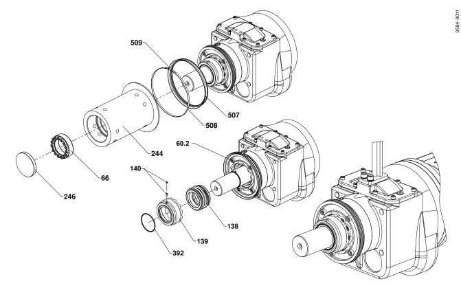
Figure 12 Mechanical seal removal/assembly XSB 2750
