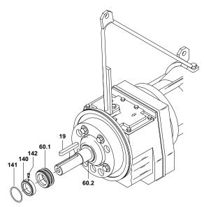
Figure 10 Mechanical seal removal/assembly SB
