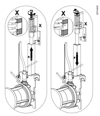
Figure 3 Locking/Unlocking of coupling system with fixed installation (Variant A)
