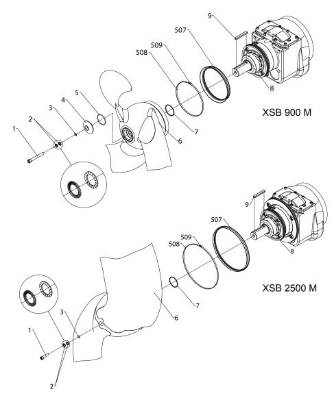
Figure 8 Mechanical seal removal/assembly XSB 900, XSB 2500
