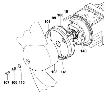
Figure 7 Propeller removal/assembly SB
