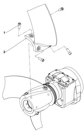
Figure 9 Propellermontage/-demontage XSB 2750
