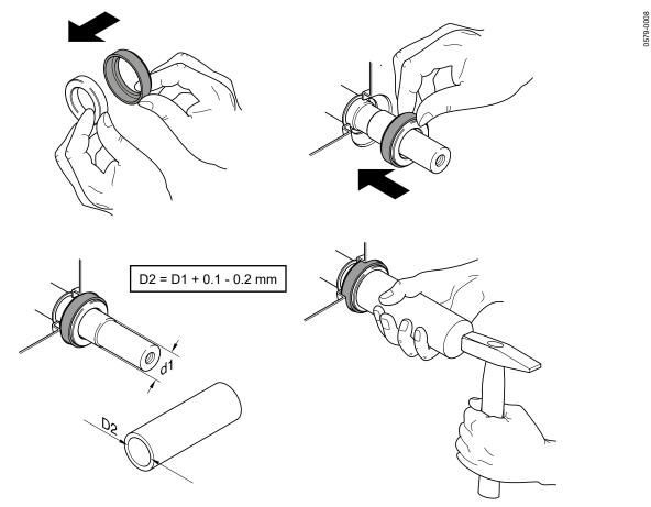
Figure 13 Fitting of the fixed ring
