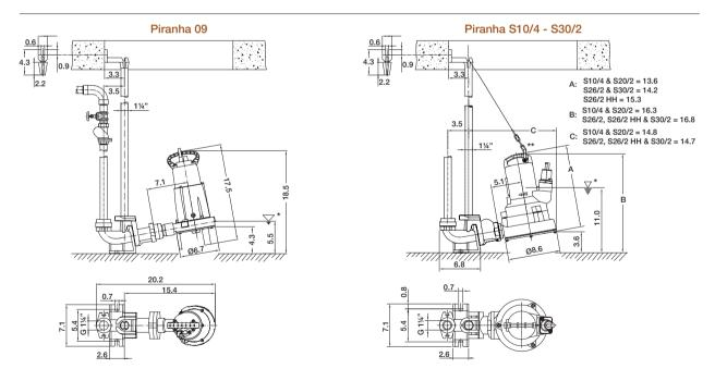
\* Lowest switch-off point for automatic operation. Minimum sump opening Ø 24.6 ins. Pedestal base secured using M10 masonry anchor bolts, drill hole size 0.6 ins.
