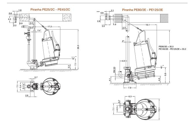
\* Lowest switch-off point for automatic operation. Minimum sump opening Ø 24.6 ins. Pedestal base secured using M10 masonry anchor bolts, drill hole size 0.6 ins.
