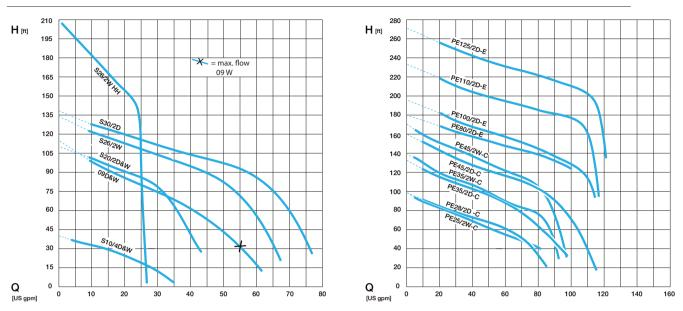
H = Total Head Q = Discharge Volume. Curves to Hydraulic Institute. N.B. please use the ABSEL program to validate pump selection.
