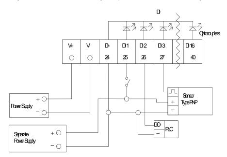
NOTE: DI- must be connected to the negative cable.
