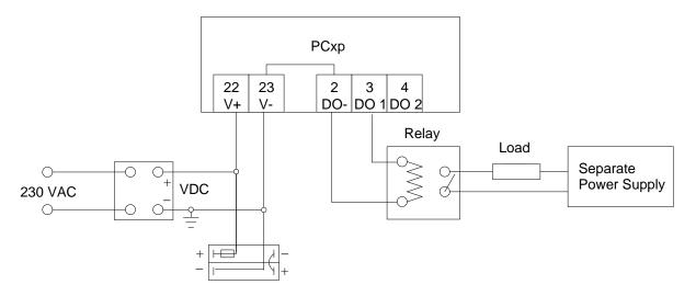
When installing a relay, The terminal number 3-10, depending on which output is used, is connected to the relay and the terminal number 2, DO-. The DO- is internally connected to V-.
