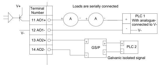
Units with a minus output connected to ground, PLC1, can be connected directly to the output. When more units are used to the same output shall these be connected serially. In the figure above is the PLC 2 not connected to the same ground as that the PCxp uses. To solve this problem, a passive galvanic isolator, GS/P, is connected between the PLC and PCxp.
