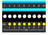
One single digital output can have a maximum current of 1 A. The total current for the 8 outputs may not be more then 4 A.
