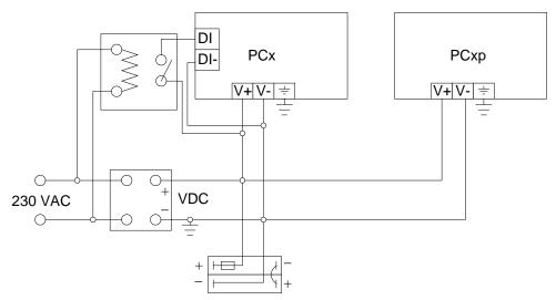
The power supply and the backup battery should be connected as the figure above. To monitor the net power, a relay can be connected to a digital input on the PCxp to receive alarm about it.
