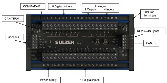
PCxp can be used in many applications. This chapter describes the most common cable wiring for the PCxp. The unit is equipped with transient and interference suppression components. When the unit is put in hazardous areas, external transient and lightning protection is recommended especially on the RS232/485-port.
