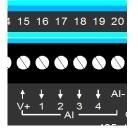
The inputs have the terminal numbers 16-19. See figure below for examples on installations. The inputs may need a galvanic isolator when connecting units to it.
