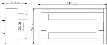
Figure 3.1: The dimensions of the PCxp when mounted on a 35 mm DIN-rail
