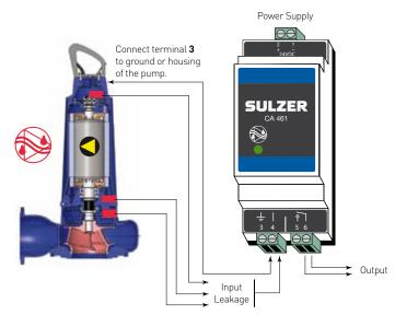
Leakage: sensors must be in parallel
