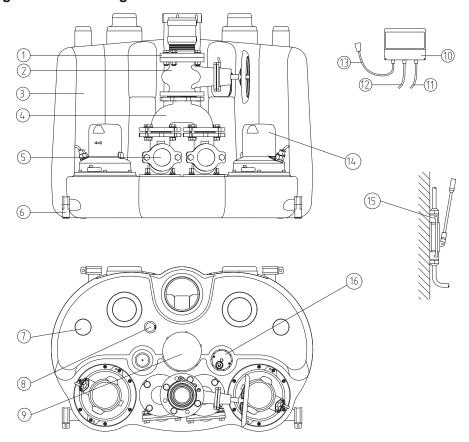
Figure 6: Design of the lifting station Sanimat 2002
