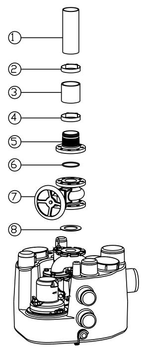
Figure 16: Installation of the shut off valve and flanged sleeve
