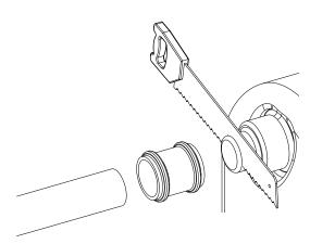
Figure 12: Opening the connections on the collection tank
