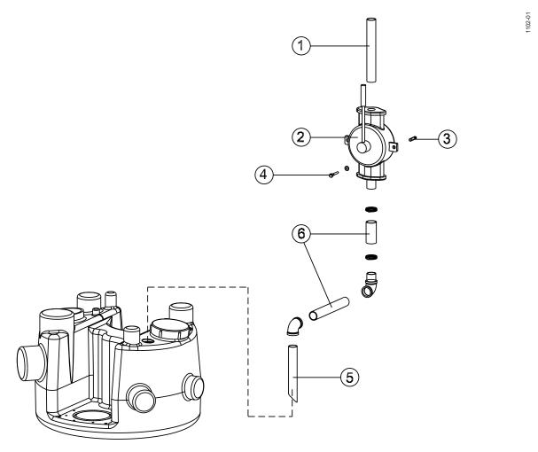
Figure 17: Installation of hand membrane pump
