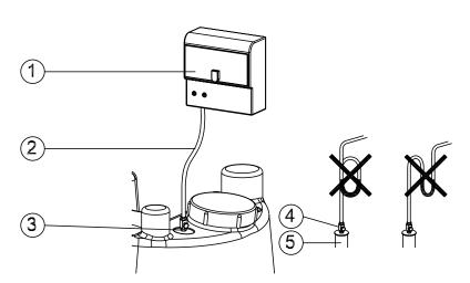
Figure 13: Installation of control line (plastic hose)
