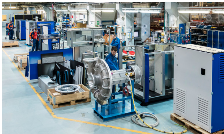
HST turbocompressors being manufactured in the Sulzer factory in Kotka, Finland.
