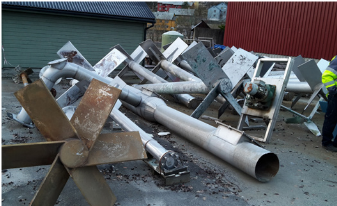
Great power savings could be achieved with Scaba hydrofoil high-efficiency impeller (below) versus pitch blade turbine (left).
