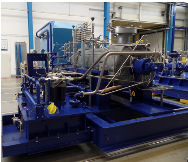
Feedwater pump in Sulzer workshop
