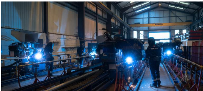
Picture 1: Boiler Tube Overlay Machines
