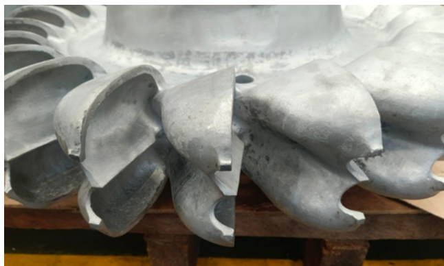
2. Bucket geometry restored through refurbishment
