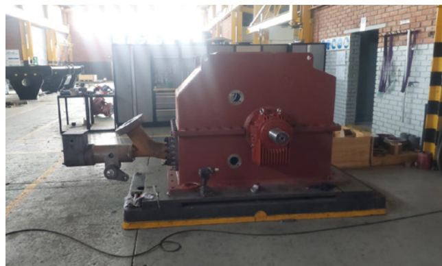
3. Refurbishment complete, ready for final coating
