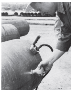
Direct contact magnetization through magnetic leech clamp of part
