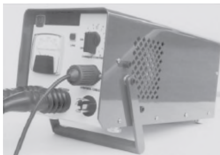
Typical portable power pack for prods
