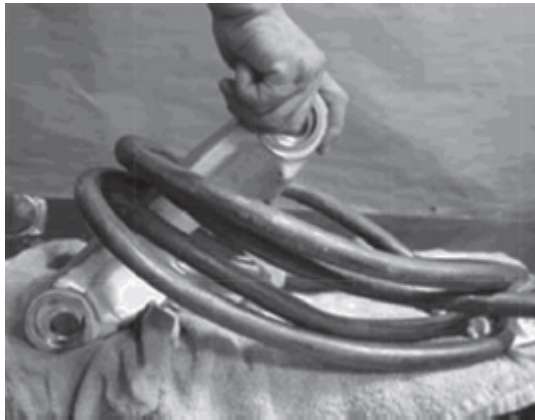
Cable Wrap Magnetization Example
