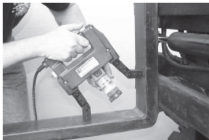
Yoke Method of Part Magnetization
