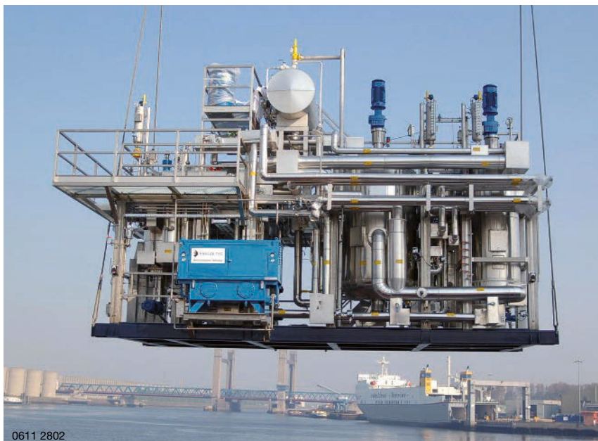
Skid mounted suspension crystallization plant for MDI
