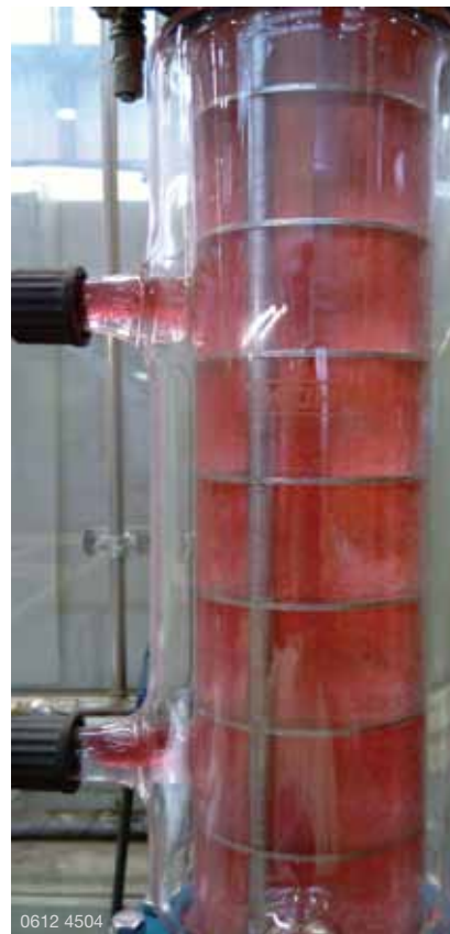
Agitated liquid-liquid extraction column in pilot scale
