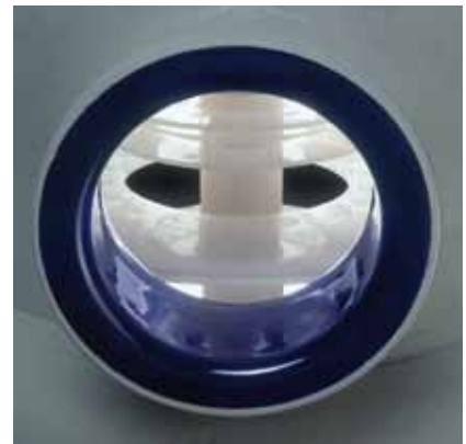
Glass-lined column shell with PVDF internals
