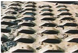
2-pass VG AF trays with V-Grid, sloped outlet weir and push valves
