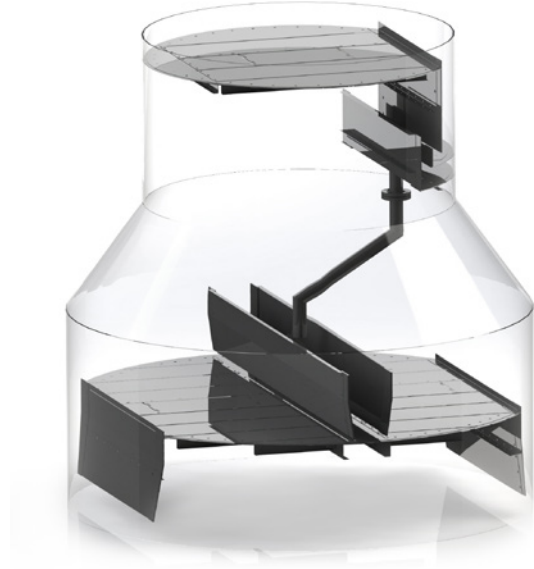
Transition from a 1-pass tray to a 2-pass tray over a conical section
