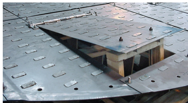
2 psi uplift BDH™ tray equipped with through-bolting assembly, shear clips and explosion doors.
