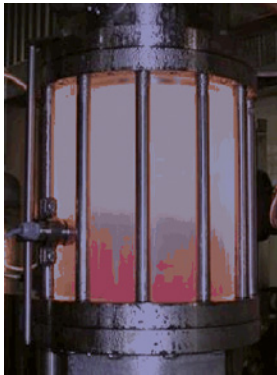
Ice separation column
