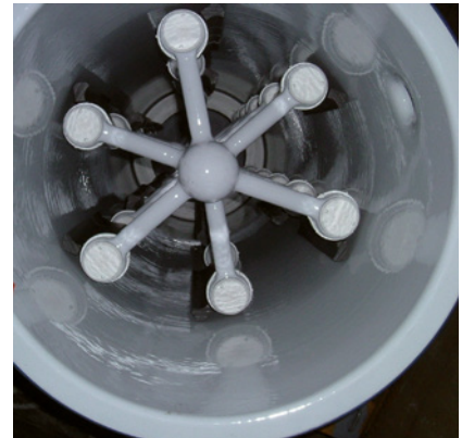
Inside of a glass-lined evaporator
