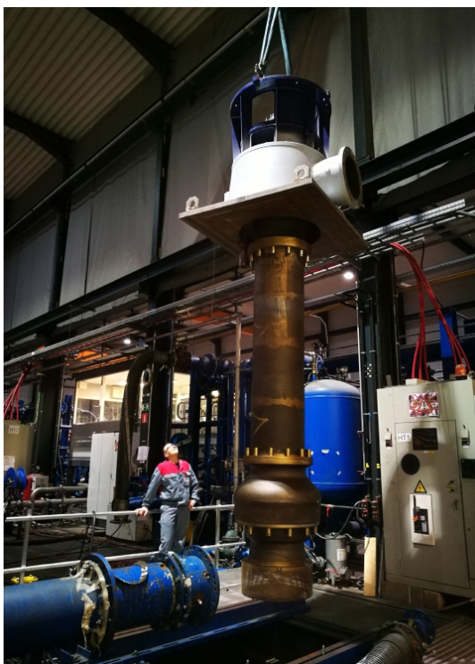
2'800 m 3 /h VAS pump on test bench
