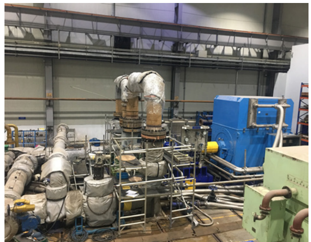
One of the feedwater pumps underwent a thermal shock test as part of the project delivery
