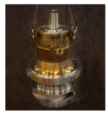
This is Sulzer's version of the primary reactor recirculation pump top end. It is used in several US BWR type nuclear power plants.
