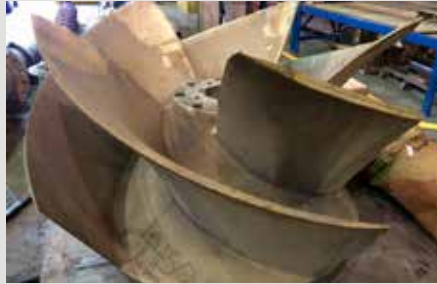
Circulating water pump impeller for power station
