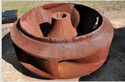
1'676 mm impeller for dewatering service
