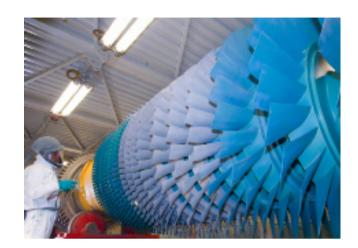
It has been shown that the surface finish of the airfoils can be satisfactorily restored by using suitable compressor coatings.
