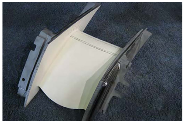
Gas turbine vane repair
