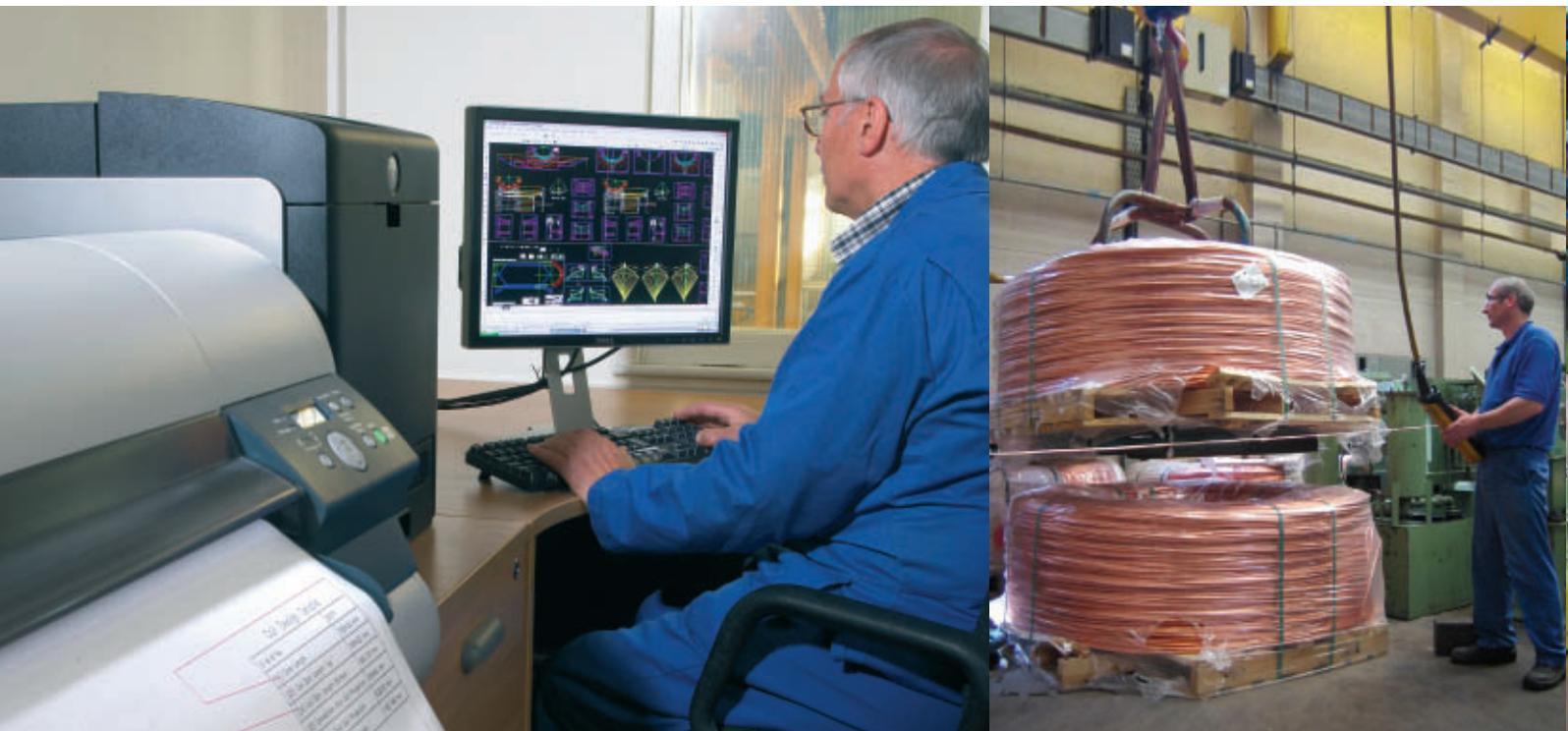
Pre-production support includes **computer aided design** and a large database of coil winding information. This enables us to check existing designs, re-design for improved performance and to produce production drawings and process instruction sheets automatically.
