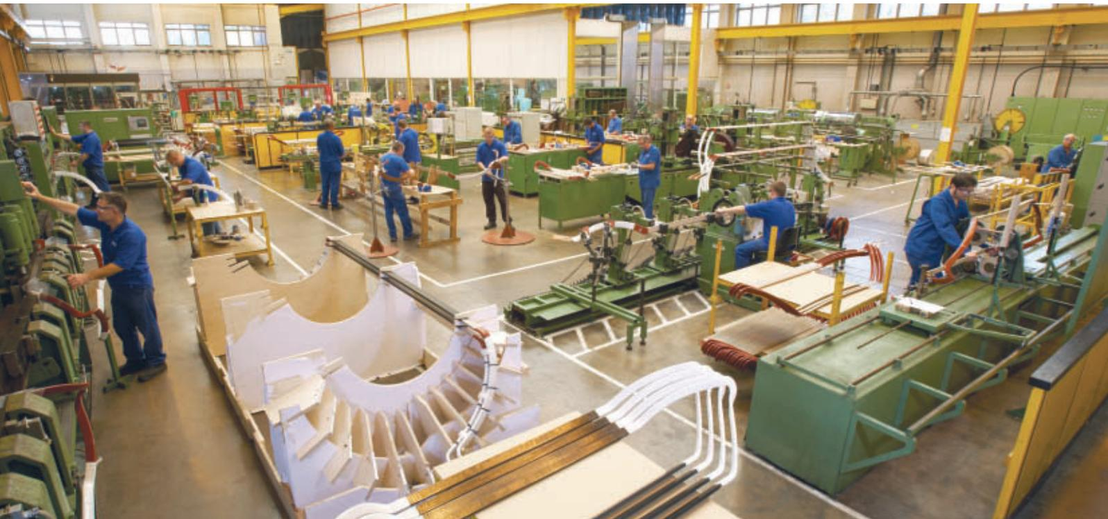
A view of the Coil Shop Incorporating a wide selection of Diamond Coils and Generator Bars.
